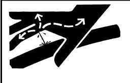
Injection Hazard: Do not try to stop a leak with your hand! Avoid any close contact with hydraulic fluid jets. Escaping fluid can penetrate skin, causing serious injury. In case of accident, see a doctor immediately for removal of fluid.
